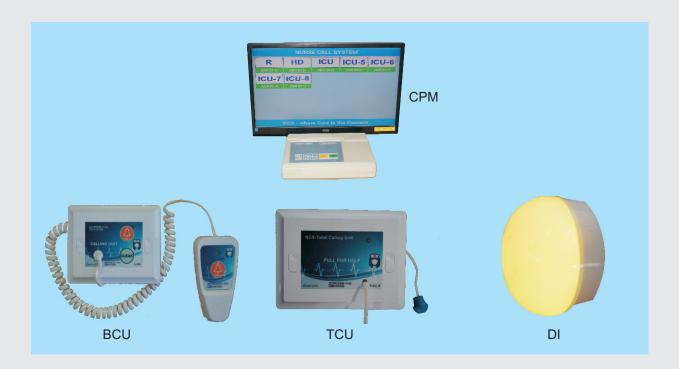
This model is designed to be very cost effective with only essential features. It can be used to upgrade existing electrical buzzer system. For new installations just a 2 pair economical cable including telephone cable can be used. One Nurse Station Display can be shared by up to 48 calling points. Makes use of very few backend communication devices apart from front end components shown in above picture.
